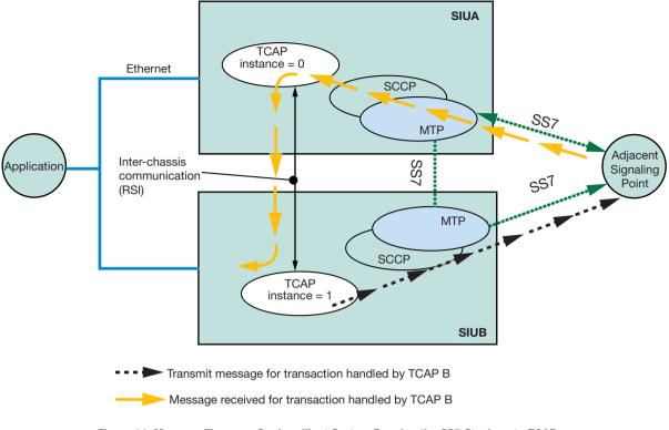
Figure 14. Message Flow on a Dual-resilient System Running the SS7 Stack up to TCAP
